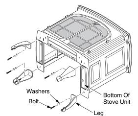
Figure 10 - Attaching Stove Legs (Oxford™ Model Shown)
